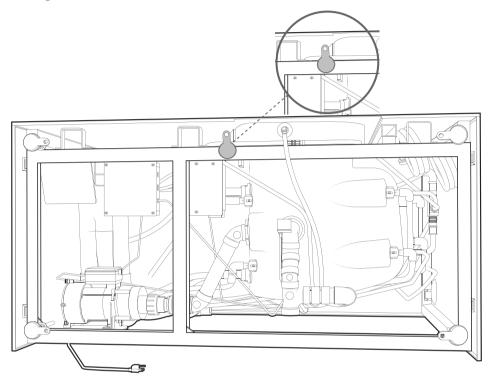
2. Do the adjustments by lowering the center foot (raise the frame) until the door can freely swing closed without rubbing on the tub, like:
