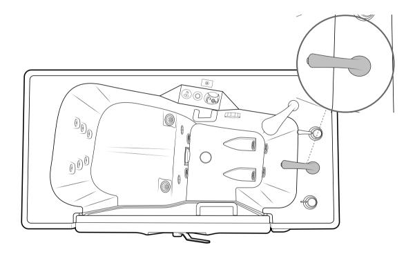
3. To drain the bathtub, turn the drain handle clockwise.
