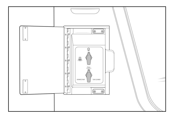
The tub has an integrated cleaning and disinfection system that pushes chemicals through the whirlpool plumbing using a Venturi injector. The 2 black knobs are used to operate the system.
