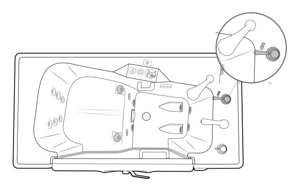
c. To turn on the fill spout turn and point the "Diverter" towards the fill spout.
