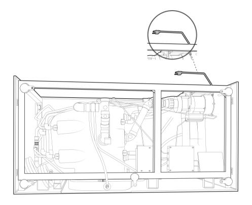
Note: The pump and inline water heater should never be plugged into the same 15A circuit.
