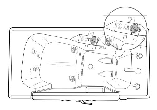
b. To increase the air flow rotate the "Jet Air Control" knob counter clockwise.
