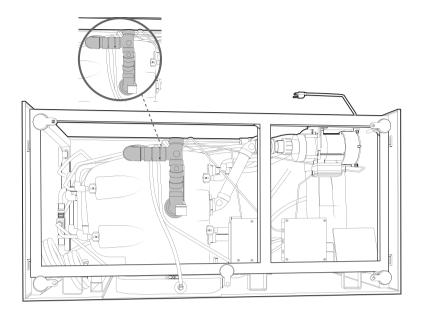
2. The drain can be attached to the building drain with PVC cement or a rubber coupler.
