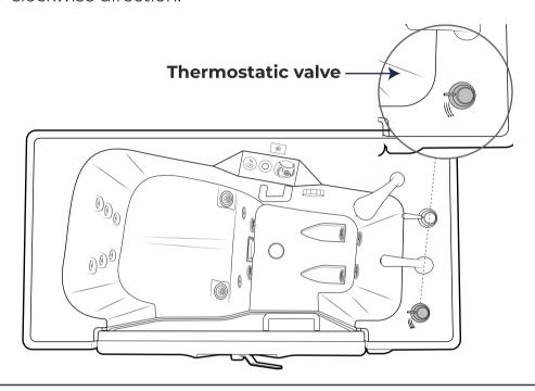
b. To decrease the temperature, turn the "Thermostatic Value" in a clockwise direction.
