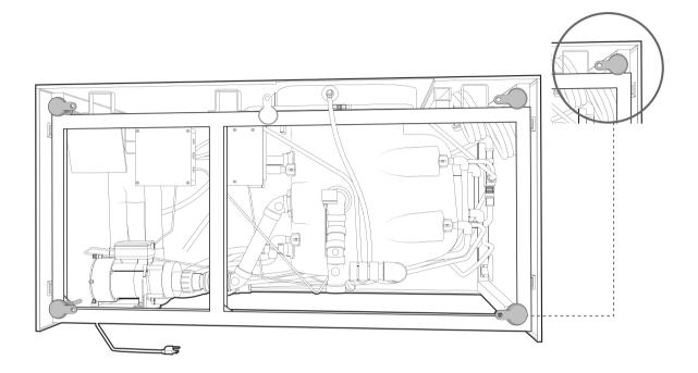
2. It is important that all of the leveling legs are completely supporting the tub and touching the floor. There must be no space between the leveling legs and the floor.
